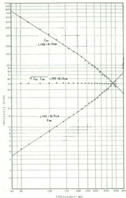
Figure 4. Open- and Short-Circuit Measurements of Air-Filled Line.
