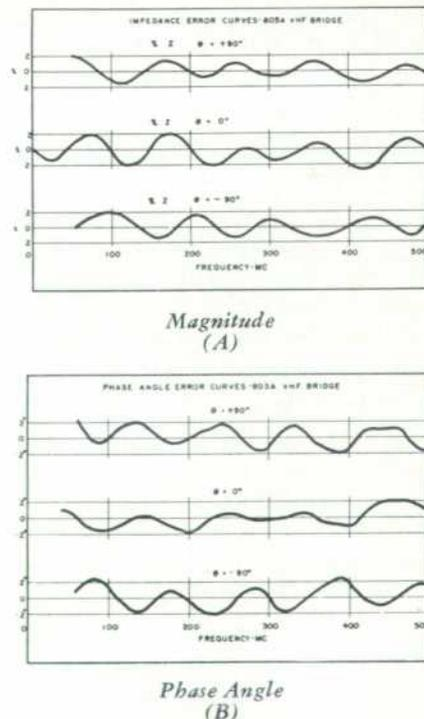
Figure 5. Typical Correction Curves Supplied with Bridge.
