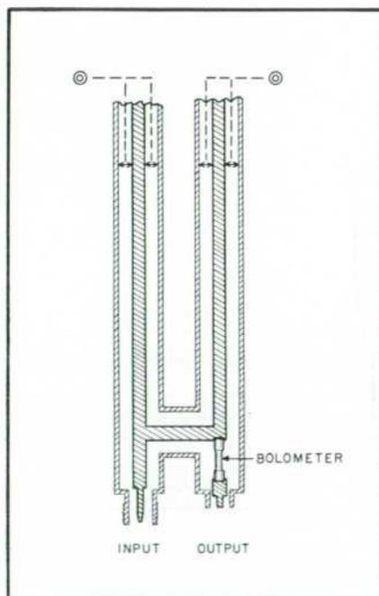
Figure 5. Cross-sectional Drawing of Tunable Bolometer Mount.
