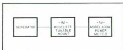
Figure 3. Set-up For Measuring High Frequency Power.
