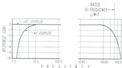
Fig. 2. Typical bandwidth characteristic of *-hp-* Model 130BR Oscilloscope. Curve applies to both vertical and horizontal amplifier and is essentially independent of sensitivity settings.
