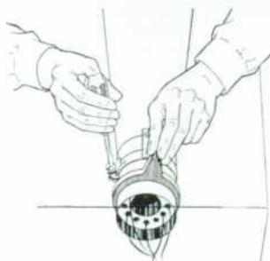
Fig. 8. Crt alignment lever simplifies angular tube positioning.
