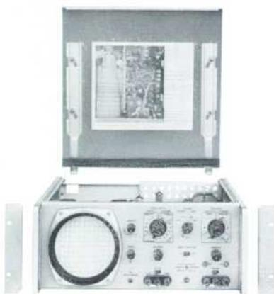
*New -hp- Model 120B oscilloscope operates from dc to 450 kc with a vertical system sensitivity of 10 mv/cm. Dual-purpose cabinet can be used either in bench service or can be rack mounted using brackets supplied. Inside of instrument top cover contains large illustration locating most components and all adjustments.*
